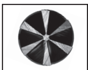
Bottom surface of 6HSS cutting edge
