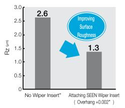
Cutting Conditions ·MSE45100R-6T-SF ·Vc = 660 sfm ·D.O.C. = 0.0079" ·Tz = 0.0039 ipt ·Dry ·No Wiper Insert SEKN42AFTN (TN100M) 6 Inserts SEKN42AFTN (TN100M) 5 Inserts SEEN42AFTR-W (TN100M) 1 Insert
