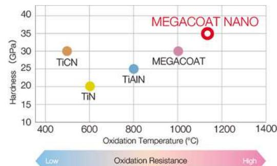
Prevents wear and fracture with high hardness (35GPa) and superior oxidation resistance (oxidation temperature: 1,150°C)
