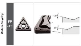
For medium to high feed with automatic lathes (when cutting medium to large diameter workpieces). Sharp Edge / Polished: Sharp Cutting. Smooth chipbreaker geometry improves chip flow with less adhesion. Large curled chips.
